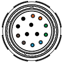
D38999 Size 11 Connector MOD Def Standard 23-04 Pinout
